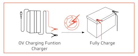
1 The charger can charge the battery starting from OV.
