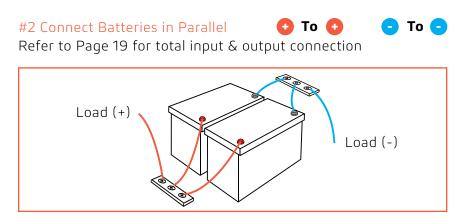
After parallel connection, the <u>capacity</u> of the battery system will be doubled according to the number of batteries you connect.
