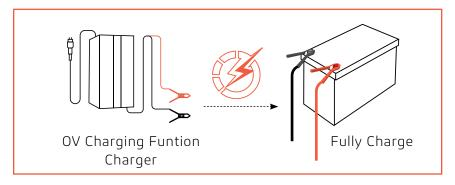
① The charger can charge the battery starting from OV.
