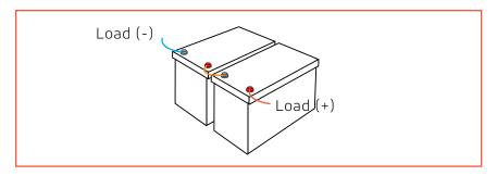
After series connection, the voltage of the battery system will be doubled according to the number of batteries you connect.
