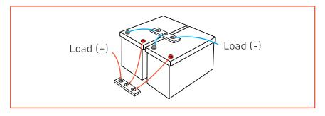
After parallel connection, the <u>capacity</u> of the battery system will be doubled according to the number of batteries you connect.
